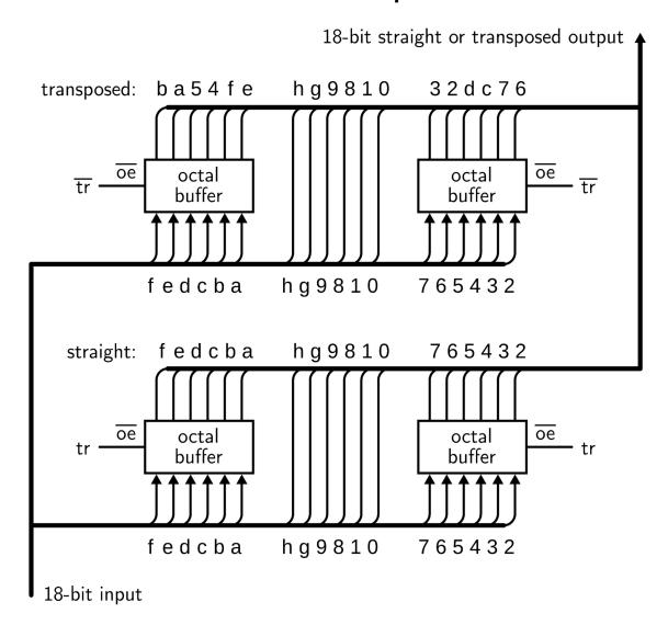
The Dauug|18 ALU has two 18-bit outputs, left and right, that each receive 6 bits from  $A_2$ ,  $A_1$ ,  $A_0$ . The left output feeds back to the left ALU operand, memory address, or memory data. The right output feeds the right ALU operand, in either "straight" or "transposed" bit order. The above diagram shows how this order is selected. (If you're curious, each octal buffer has two unused bits.)
