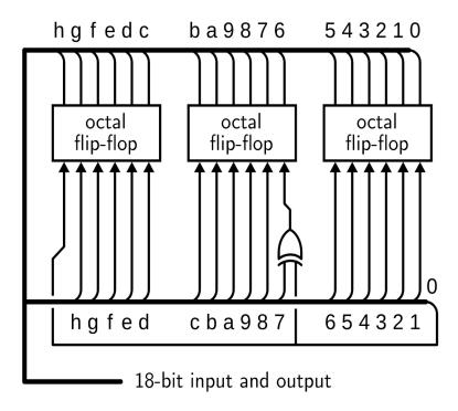
The Dauug|18 instruction pointer is an ordinary Galois linear feedback shift register (LFSR) with feedback taps at bits 6 and 17 and period 262,143. The main thing to note is that the flip-flop outputs can be disabled, which allows an adjacent bus transceiver to change the program counter during branch instructions. (If you're curious, each octal flip-flop has two unused bits.)
